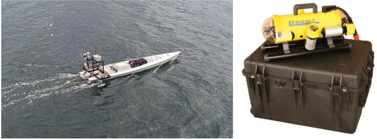
Figure 1: Methods of Data Collection USV Hydrographic Survey and ROV Inspection
